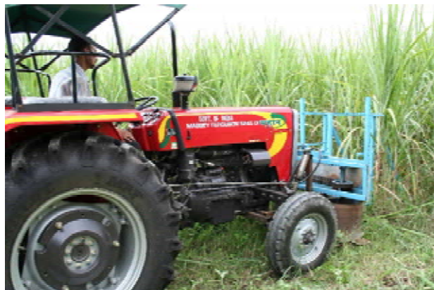
Fig. 7.1: Tractor operated front mounted sugarcane harvester in operation
