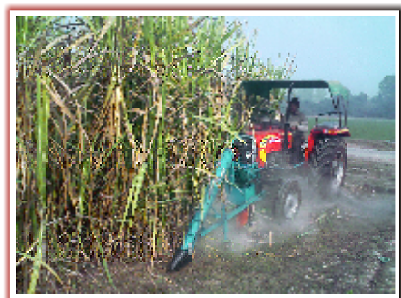
Fig. 3.6: IISR tractor operated sugarcane harvester in operation in wide spaced paired row (30:120 cm) cane crop
