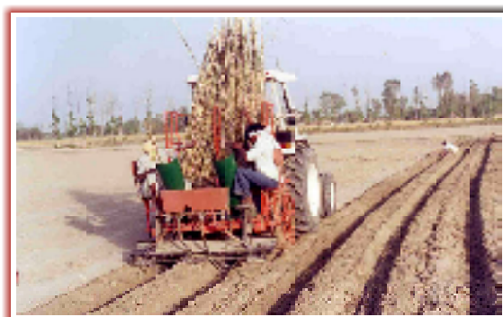
Fig. 18.2: IISR tractor operated RBS Cane Planter in operation
