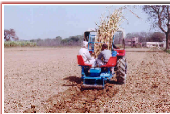
Fig. 18.4: IISR tractor operated paired row sugarcane planter in field operation
