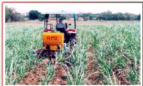
Fig. 18.1: IISR tractor operated ratoon management device infield operation
