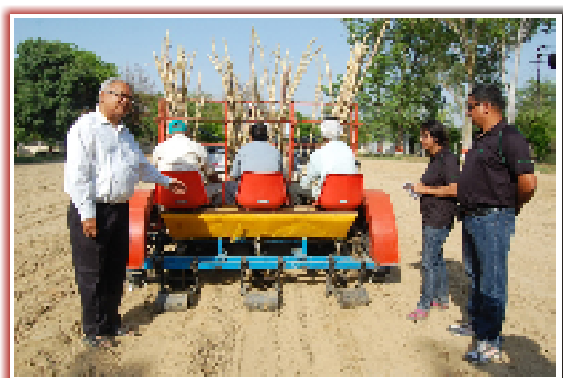
Fig. 18.3: IISR tractor operated modified three row sugarcane planter in field operation
