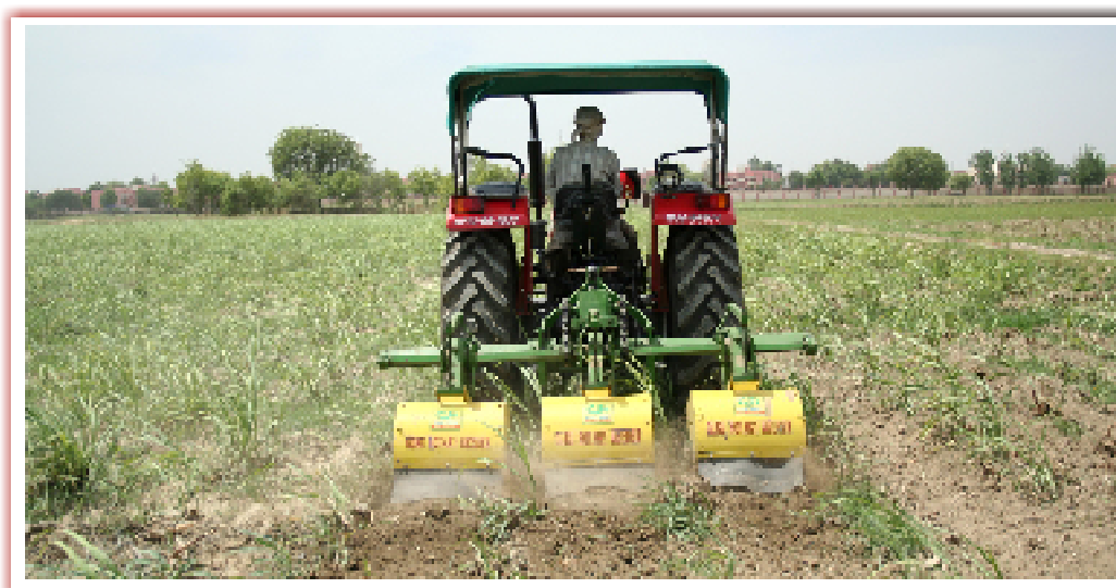
Fig. 3.7: Tractor operated three row rotary weeder in field operation at IISR farm
