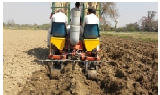
Fig. 5.2 Deep furrow sugarcane planter with herbicide spraying attachment
