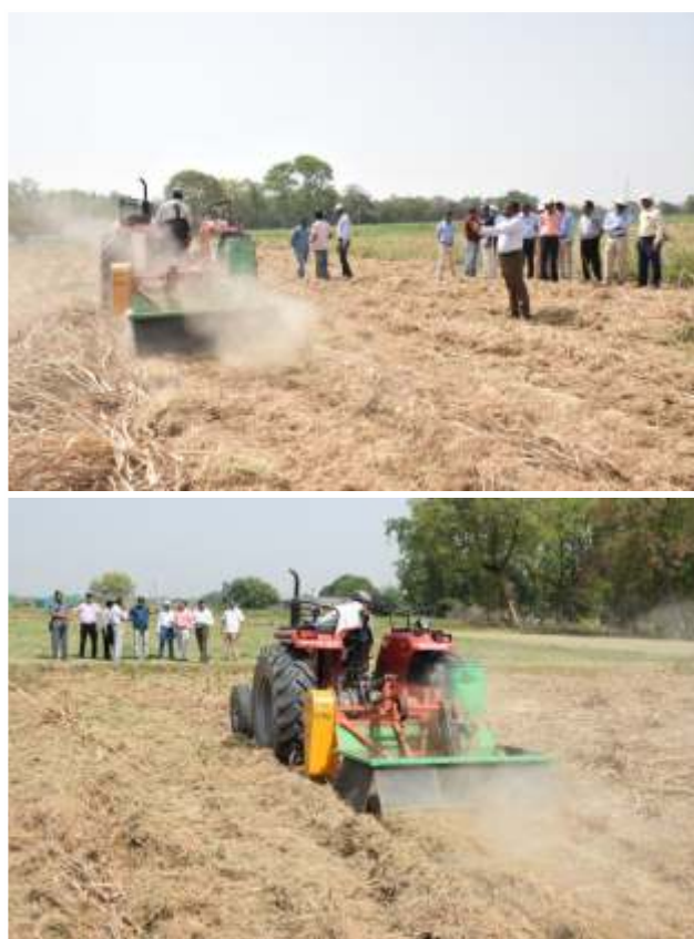
Fig. 5.2 Testing of tractor-operated trash mulcher-cum-stubble shaver device
