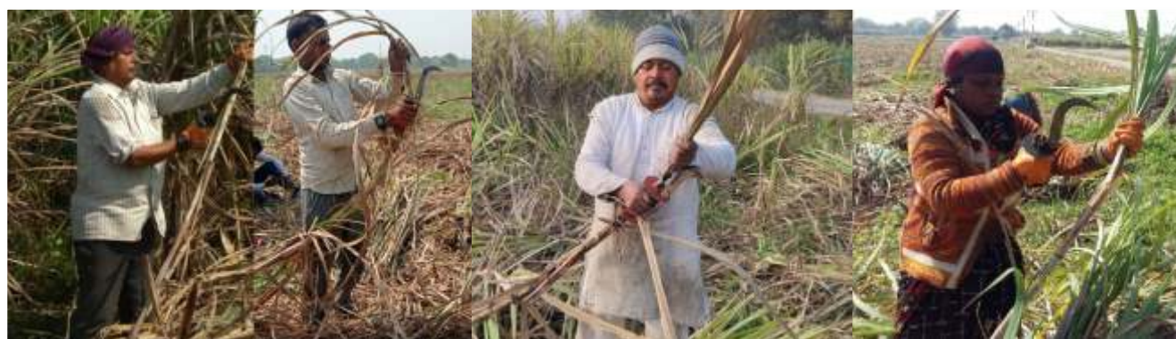
Fig. 5.4 Testing of newly developed manual sugarcane stripper-cum-detopper
