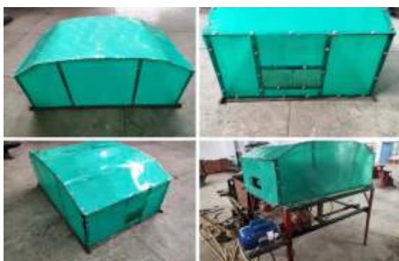
Fig. 6.1 Safety/protective cover provided on sugarcane cleaner-cum-washer
