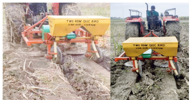
Fig. 5.17 IISIR tractor operated two row disc type ratoon management device in field operation
