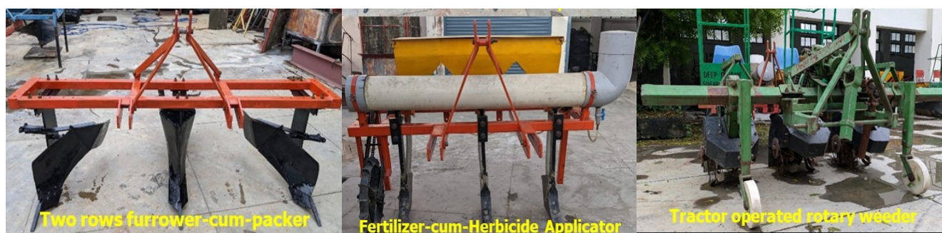
Fig. 5.3 Fabrication of matching implements for various farm operations in the field for CTF
