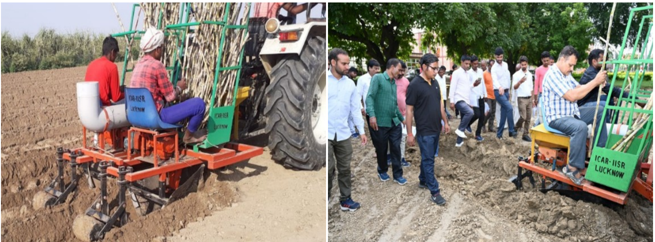
Fig. 5.16 IISIR tractor operated modified deep furrow sugarcane planter in field operation
