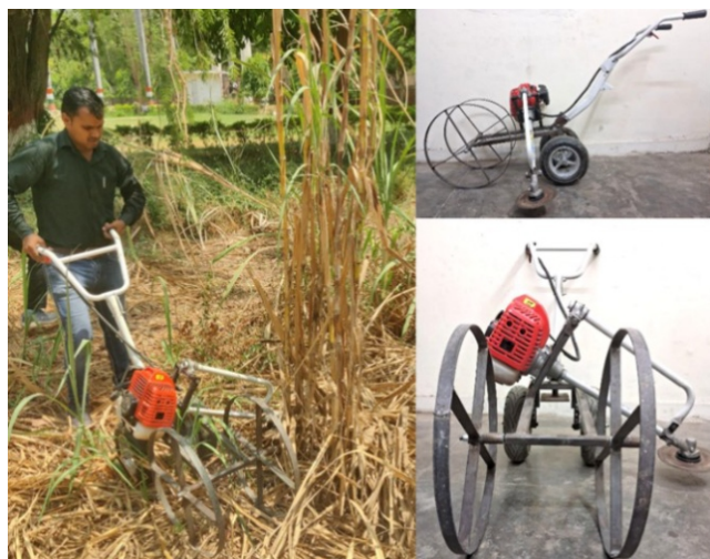
Fig. 5.12 Development of small harvesting system for sugarcane
