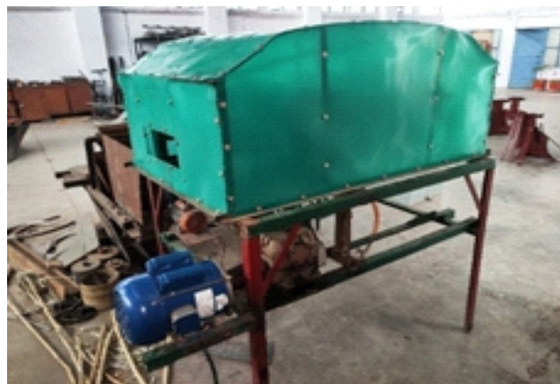
Fig. 6.1 Sugarcane cleaner-cum-washer with protective /safety cover
