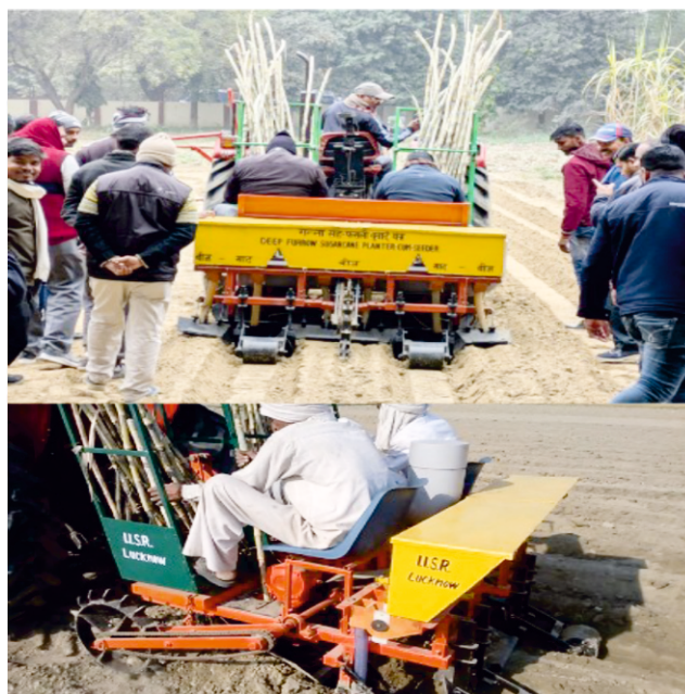
Fig. 5.18 IISR Tractor Operated Deep Furrow Sugarcane Cutter Planter -Cum- Multicrop Raised Bed Seeder in field operation
