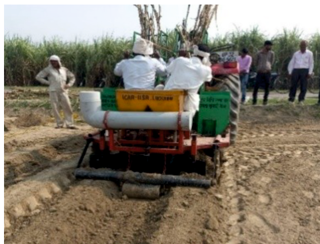
Fig. 5.10 Automatic potato-cum-sugarcane trench planter under field operation
