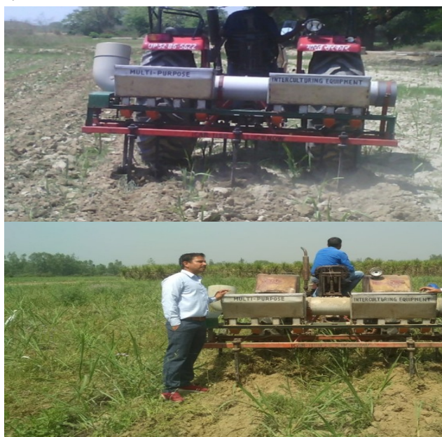
Fig. 5.19 IISR Tractor operated multipurpose interculturing equipment in field operation
