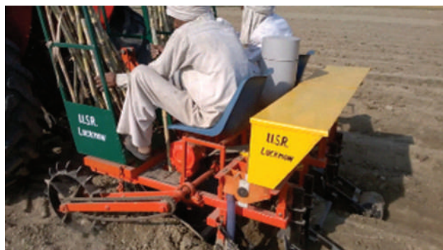
Fig. 5.17. ISRI Tractor Operated Deep Furrow Sugarcane Cutter Planter -Cum- Multicrop Raised Bed Seeder in field operation
