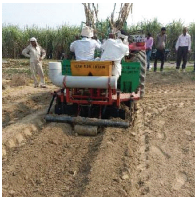
Fig. 5.12 Automatic potato-cum-sugarcane trench planter under field operation
