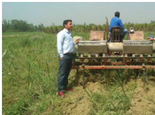
Fig 5.18. Multipurpose interculturing equipment in field operation
