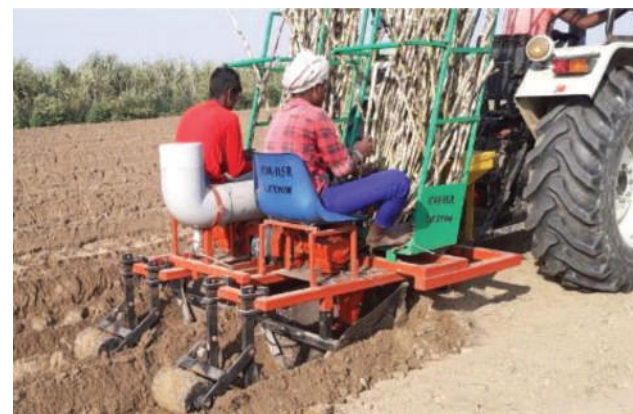
Fig. 5.15. ISRI tractor operated modified deep furrow sugarcane planter in field operation
