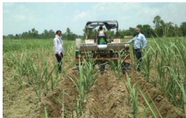
Fig 5.19. Multipurpose interculturing equipment during earthing up mode
