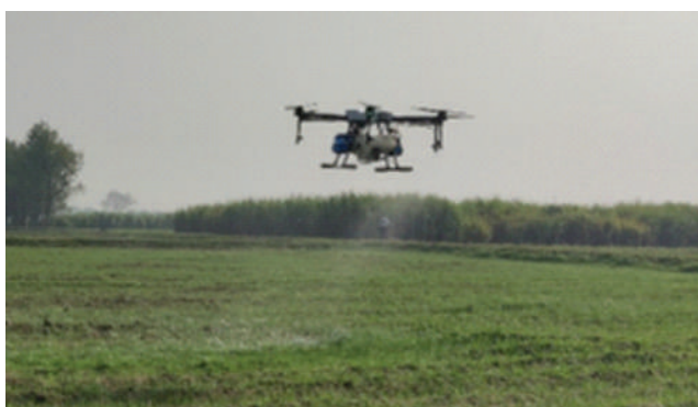
Fig. 5.13 Drone for spraying of agro-chemicals under field operation
