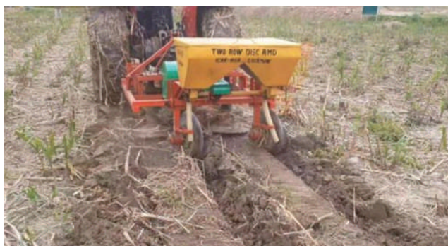
Fig. 5.16. ISRI tractor operated two row disc type ratoon management device in field operation
