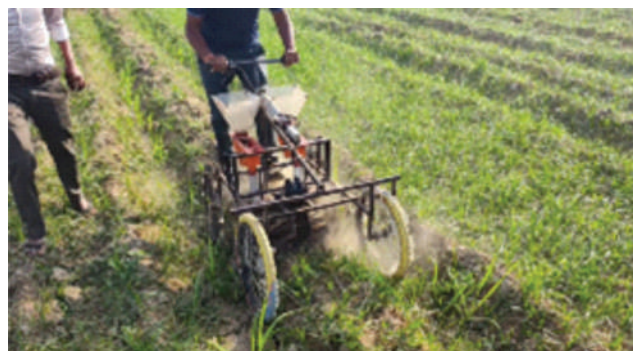
Fig. 5.14. A view of working of E-powered weeder cum seeder for intercropping in sugarcane
