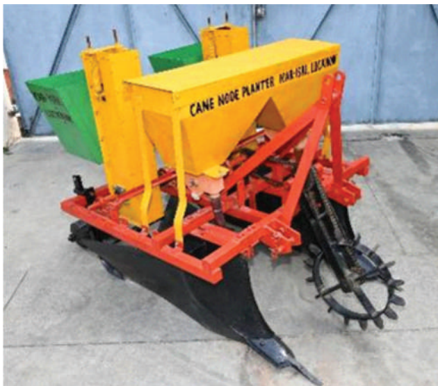
Fig. 5.1 Tractor operated cane node planter with modified cane metering mechanism
